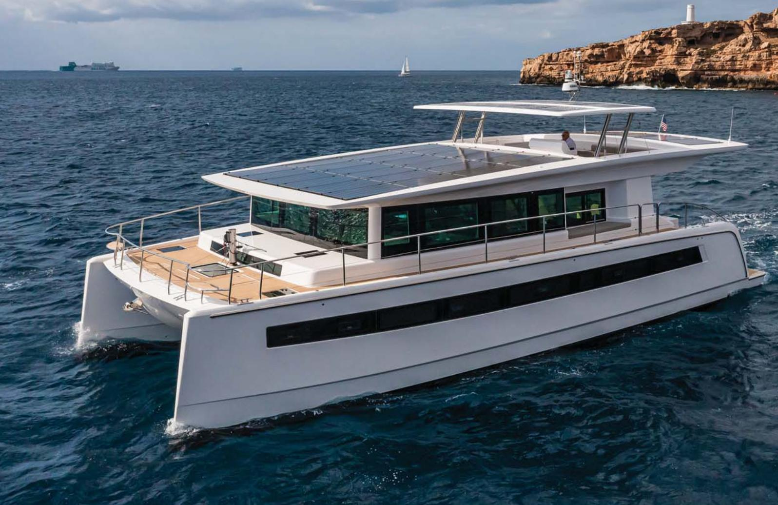
The Silent 60 is the first in a new wave of models by Silent designed by Pattaya-based Dr Albert Nazarov and constructed in nearby Rayong by PMG Shipyard. The Silent 60 is a true bluewater vessel that offers a cruising speed of 6-8 and features 42 powerful 17kWp solar panels on the roof of the superstructure and flybridge
