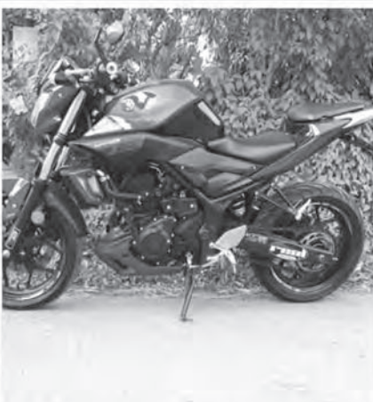
Small size sport style naked bike. 321 cc, 2 cylinder, 42 BHP, max speed about 190km/h
